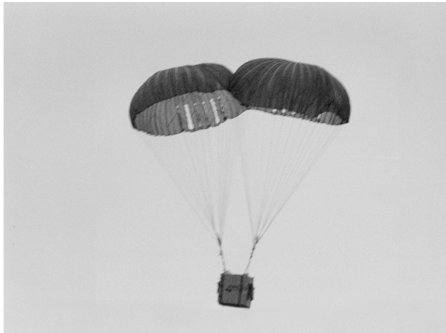
Fig. 6 Photograph of a cluster of two connected one-quarter-scale G12 parachutes during a turn.
