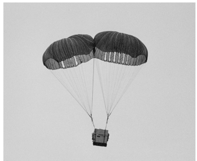
Fig. 4 Photograph of a cluster of two connected one-quarter-scale G12 parachutes during steady glide.
